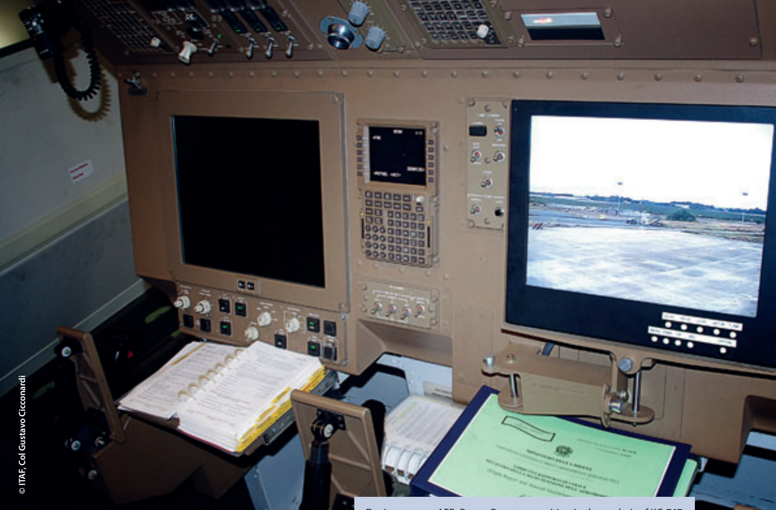
Decimomannu AFB. Boom Operator position in the cockpit of KC-767.
