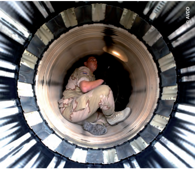
F-16 exhaust inspection at deployed location.
