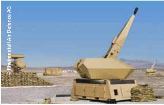
Figure 2 – An unmanned search and tracking sensor unit (l.) and an unmanned gun (r.) of the Skyshield Air Defence System.
