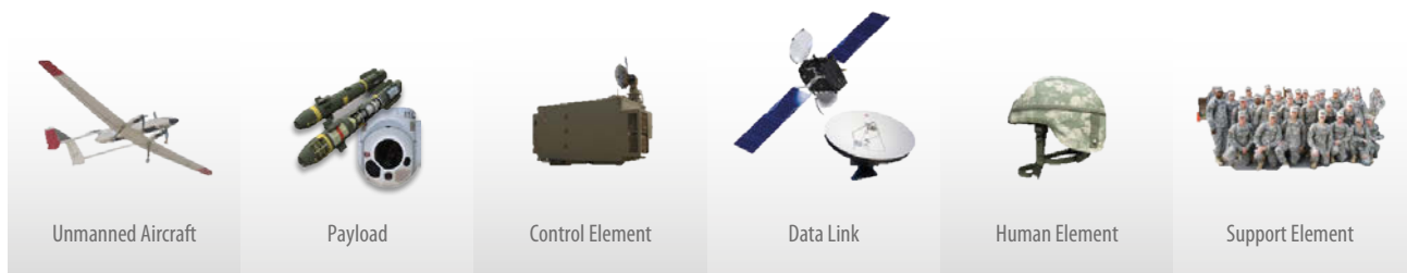
Figure 1: Unmanned Aircraft System Components.
