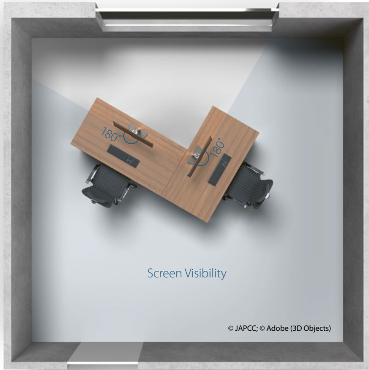
Figure 12: Avoiding the Line of Sight between Window and Screens.
