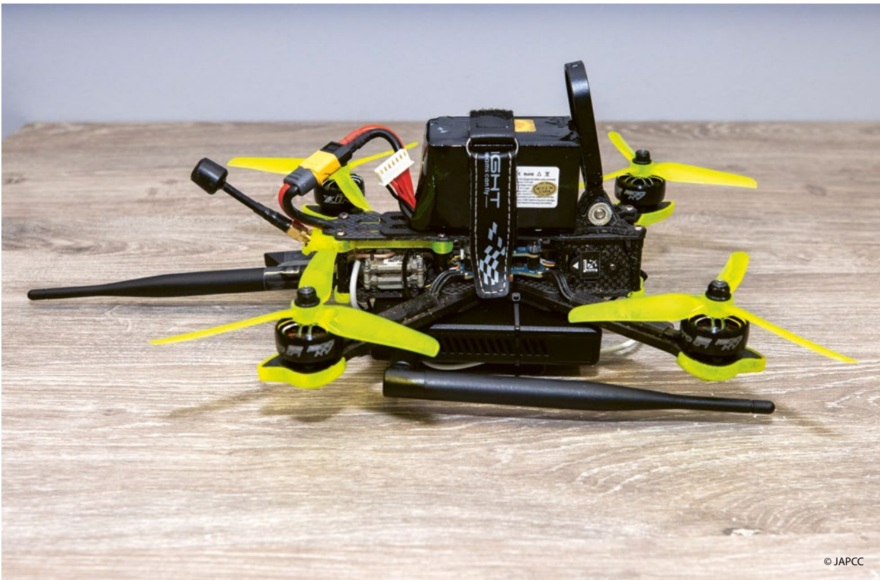
Figure 18: The WiFi Pineapple mounted below a small customized drone.
