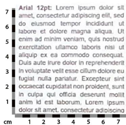
Figure 8: Image Taken with an iPhone 12 Pro with Double Optical Zoom at a Distance of 2 m.
