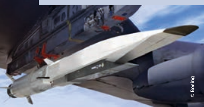
US X-51 – Hypersonic SCRJ powered experimental vehicle
