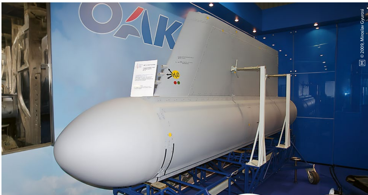
Russian SAP-14 escort jamming pod on display – designed for Su-34/35 to disrupt enemy radar.
