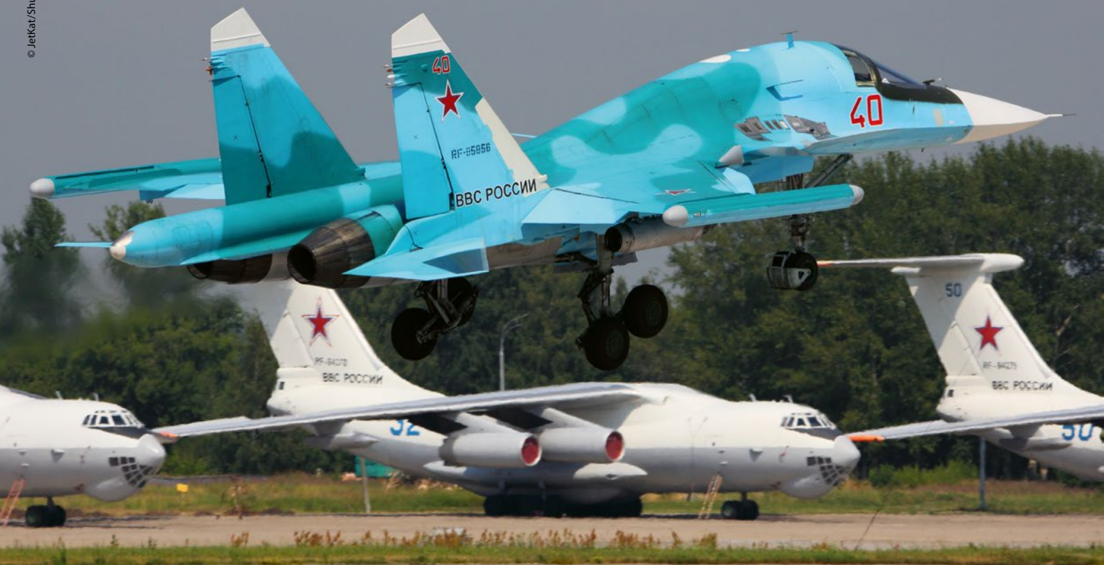
A Russian Su-34 takes off with electronic countermeasures on the wingtips.
