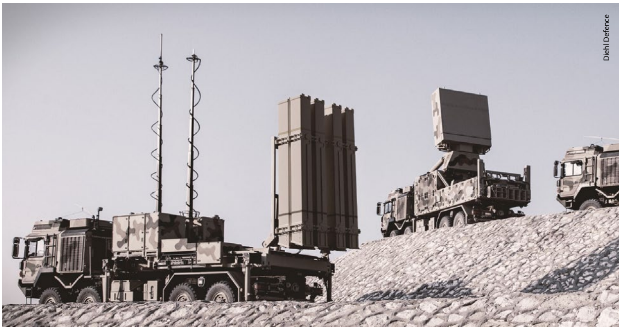
German IRIS-T SLM air defence system – capable of countering aircraft, missiles, and drones with networked radar and ECM resistance, posing a serious challenge to Russian EW assets.
