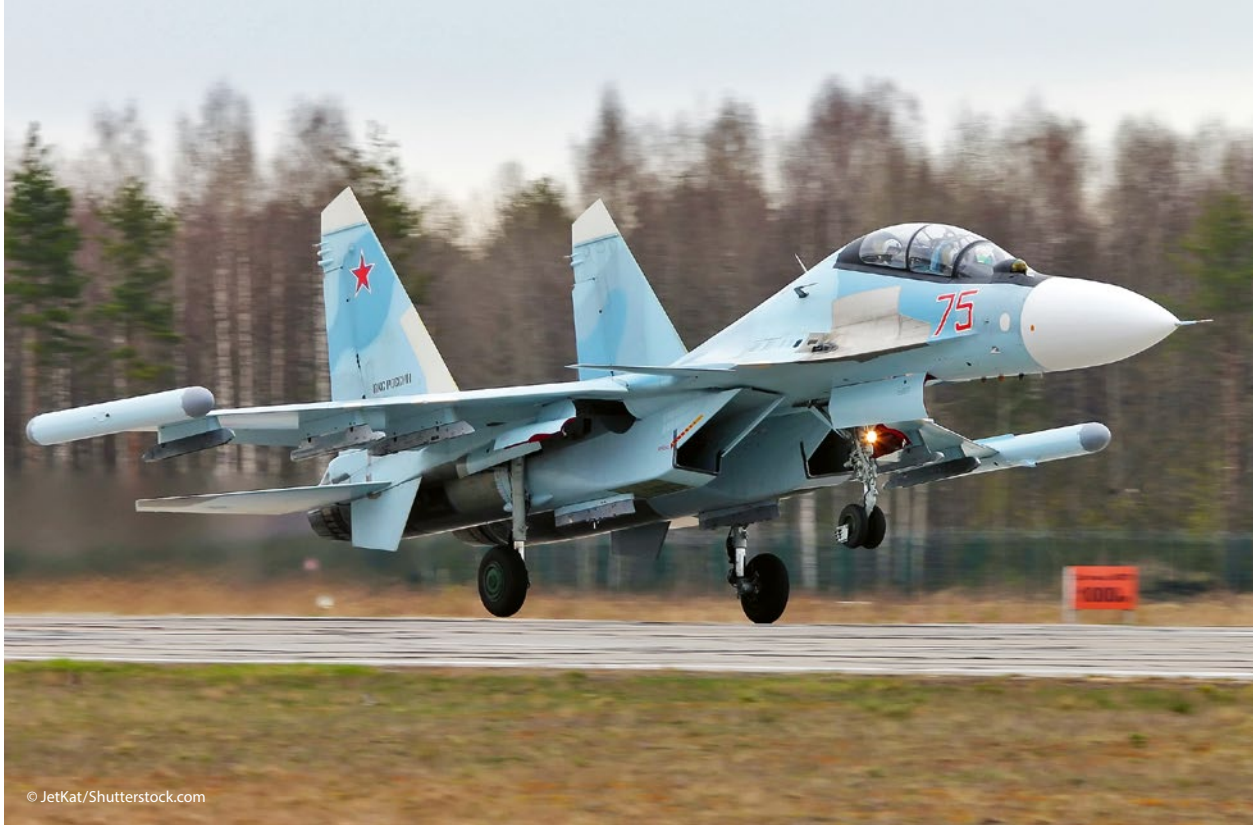
A Russian Su-30SM fighter outfitted with wingtip-mounted Khibiny-U EW pods.
