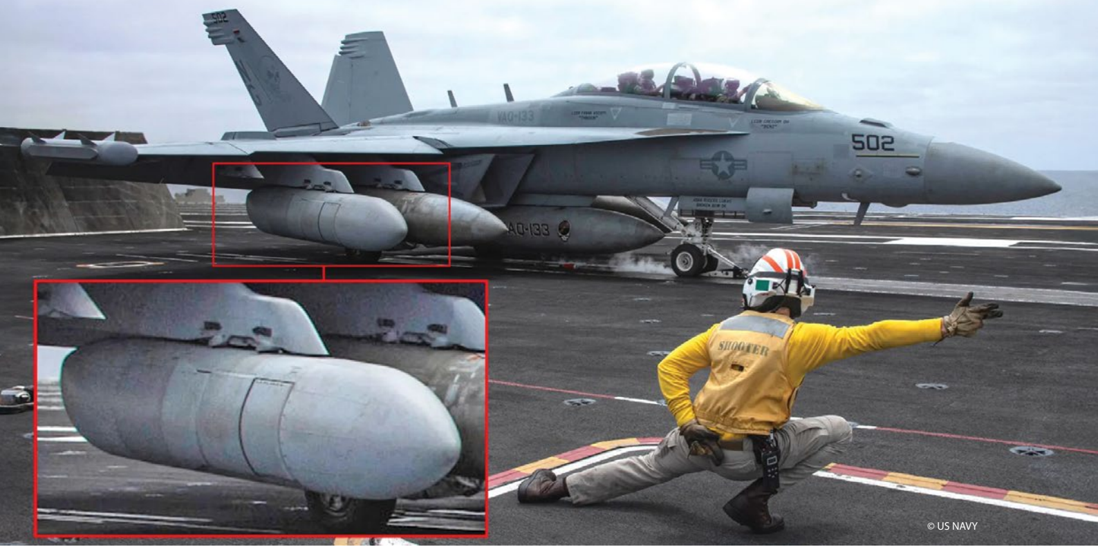
An EA-18G Growler with AN/ALQ-99 pods on the deck of the USS Abraham Lincoln.
