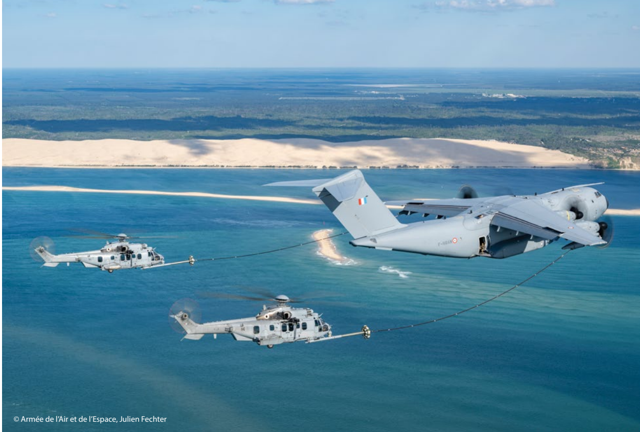
Air-to-Air Refuelling of two Caracals by an A400M Atlas assigned to special operational forces. This capability required pilots to develop advanced skills through a dedicated and targeted training programme.
