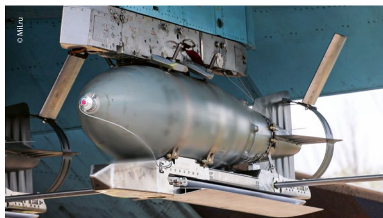
FAB-500T with a UMPK kit under the wing of a Su-34.
