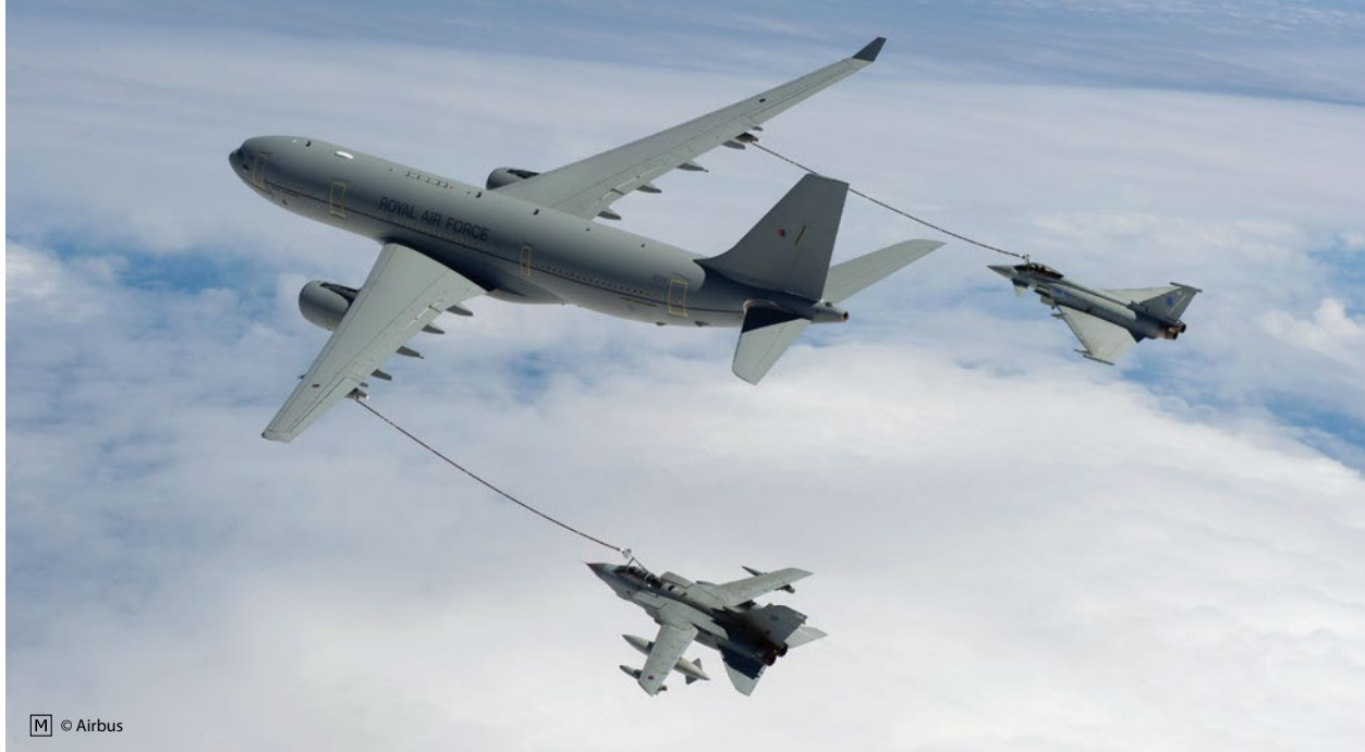
An A330 Voyager simultaneously refuels a Eurofighter Typhoon and a Tornado using the probe-and-drogue system, highlighting the flexibility and efficiency of multi-aircraft refuelling.
