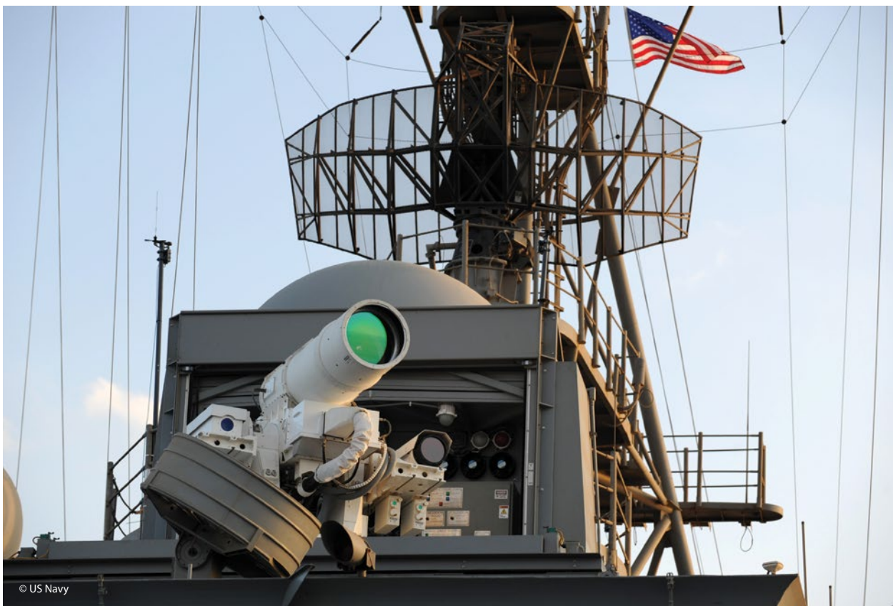
The US Navy demonstrates the Laser Weapon System (LaWS) HEL during operations in the Arabian Gulf.
