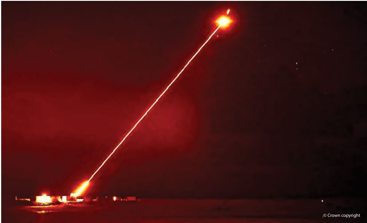
The DragonFire HEL fires during a trial at the UK Ministry of Defence Hebrides Range, January 2024, marking the UK's first high-power laser firing against aerial targets.
