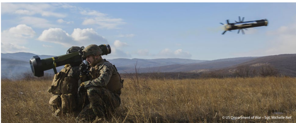
A Javelin anti-tank guided missile launches from its firing post. Weapons designed to defeat armoured vehicles have seen use against low-flying aircraft
