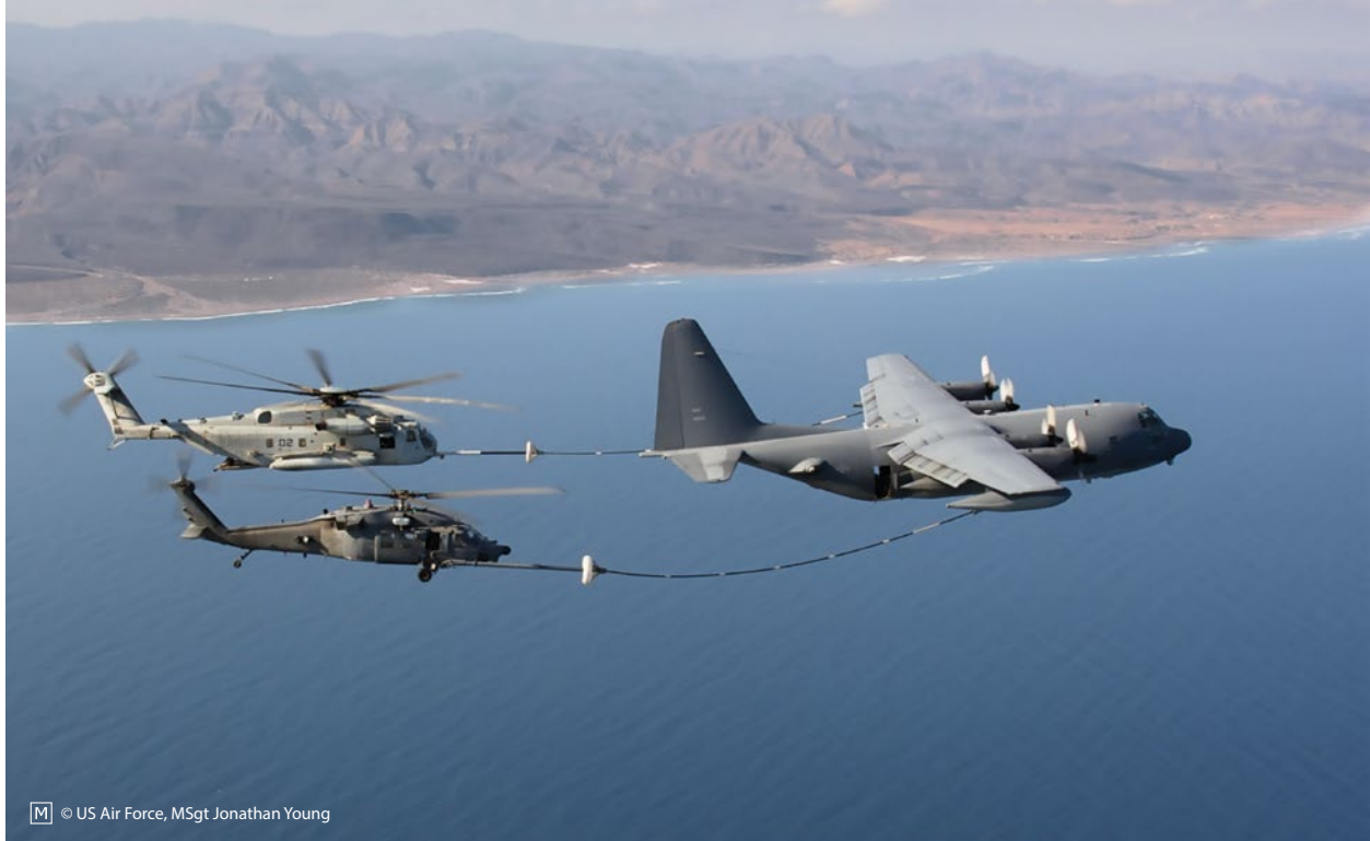
A US Marine Corps CH-53 and USAF HH-60 conduct aerial refuelling with an MC-130 assigned to Combined Joint Task Force – Horn of Africa, demonstrating that refuelling capability exists beyond the rear echelon.
