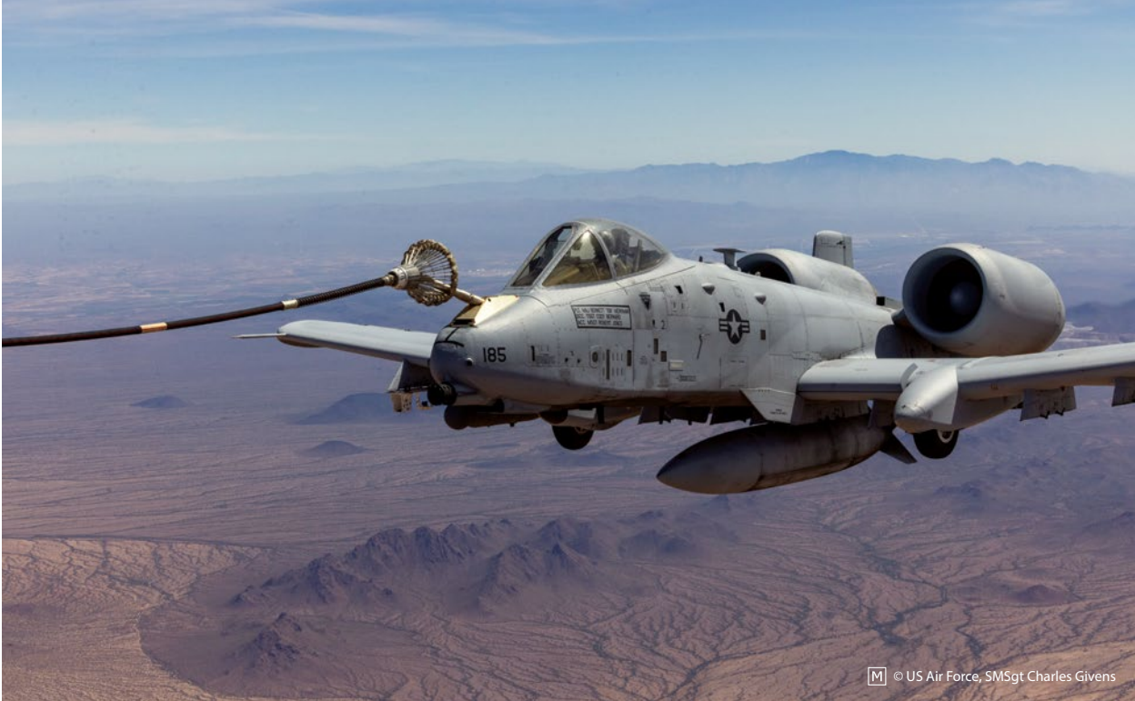
An A-10 Thunderbolt II receives fuel using the probe-and-drogue method during an AAR exercise over a desert landscape.
