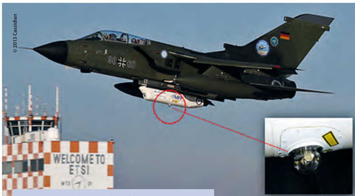
Figure 2: MLT as pod integrated solution for Air-to-Ground LaserCom.
