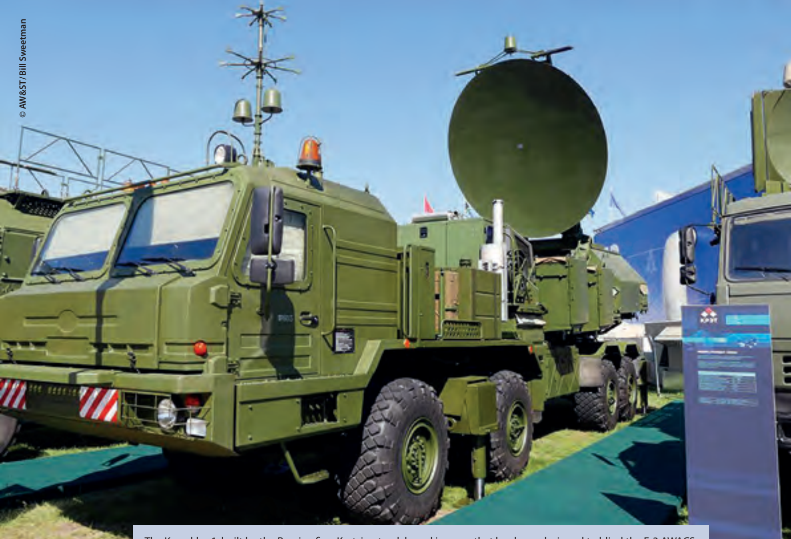
The Krasukha-1, built by the Russian firm Kret, is a truck based jammer that has been designed to blind the E-3 AWACS.
