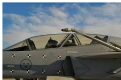
2) JAS-39 D: The probe's tip position in extended position is between the first and the second seat.
