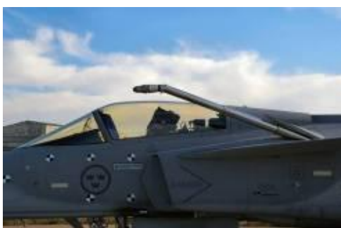
1) JAS-39 C: The probe tip in extended position (204cm plus 38cm probe tip) is at the level of the pilot's seat.
